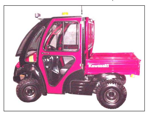
This cab is shown with the following optional equipment: hard sided doors, work lights, windshield wiper, strobe light, and antenna for overhead console. Other options not shown are: soft sided doors and an anti-draft panel for underneath the bench seat.
